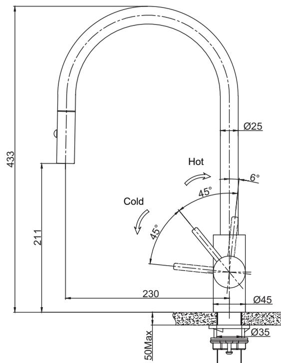
**PLEASE NOTE:** Large and heavy taps should ideally be mounted directly through the solid benchtop or fully supported from underneath. For all other swivel taps, we recommend the use of the Franke Tap Support Arm to provide additional support. Please ensure all Franke tapware is installed at a pressure of no greater than 500 kPa in accordance with AS/NZS3500 and insist that your plumber flushes all of the water supply lines before installing tapware. Failure to do so may void warranty.
